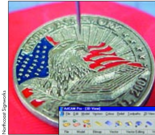
The original design for the Memorial emblem came from a lapel pin. Jim and Bill Hamilton of Northcoast Signworks scanned the pin and transferred the image to their router where they carved the original two-foot emblem from HDU.
