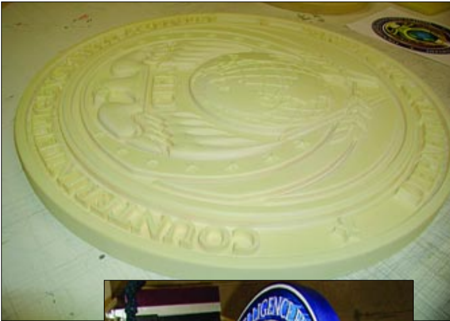
This HDU emblem is 24" around and 2" thick. McMahan painted it with an airbrush. It was clear coated so visitors can touch it.
