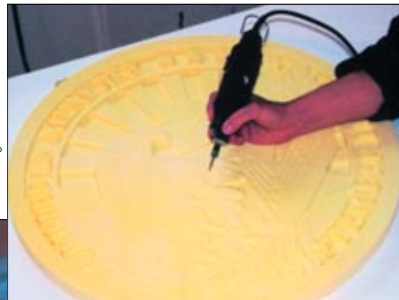
Once the piece was routed, McMahan went back over it, "sharpening up" the image by hand.
