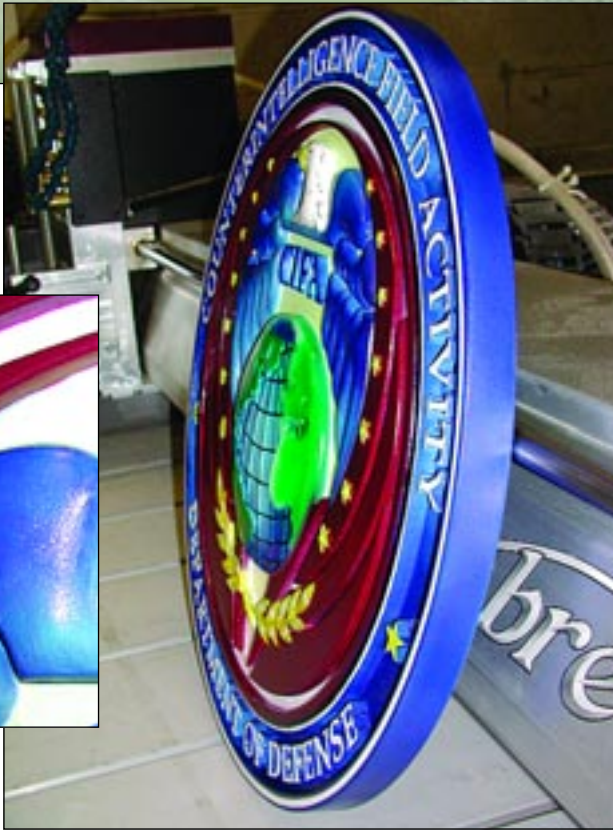
This HDU emblem is 24" around and 2" thick. McMahan painted it with an airbrush. It was clear coated so visitors can touch it.
