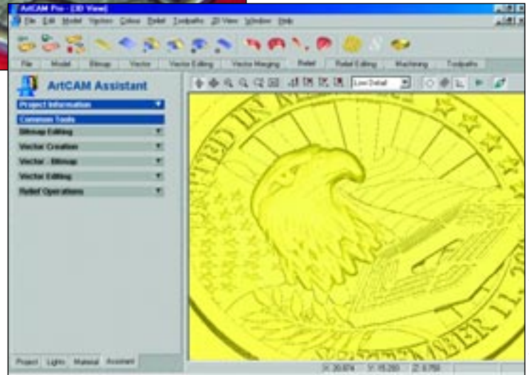
The original design for the Memorial emblem came from a lapel pin. Jim and Bill Hamilton of Northcoast Signworks scanned the pin and transferred the image to their router where they carved the original two-foot emblem from HDU.
