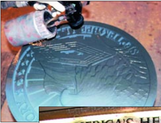
The cast emblem was sent to LuminOre where it was sprayed with an aluminum metal composite.
